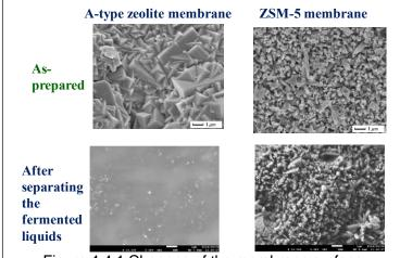
Figure 4.4.1 Changes of the membrane surface morphology after treating the fermented liquids
