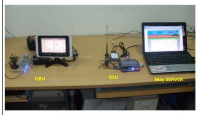
These devices support to monitor vehicles on the road using GPRS, GPS systems. Position and speed of vehicles are sent to server. An administrator can view the information of each vehicle as well as seeing the traffic photos taken by the
